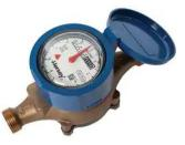
Check for leaking pipes by reading your meter before and after a two-hour period when no water is being used. If the readings are different, you have a leak.
